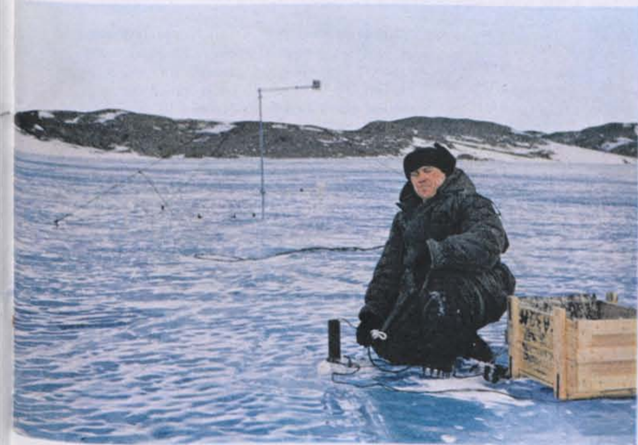
Nikolai Grigoryev, an expert on frozen soil, measures below-the-surface temperatures at Bunger Hills, a Soviet scientific substation about 200 miles from the main base.
