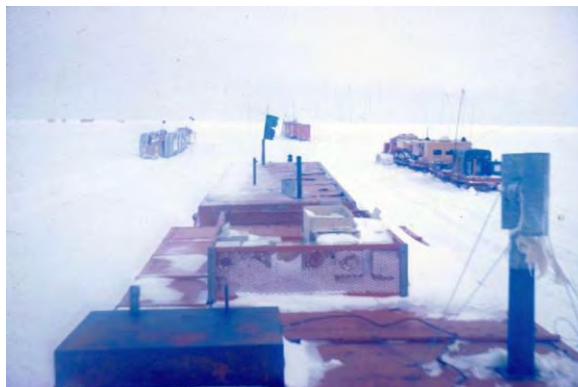
Greenland "swing." Wanigans, large sleds, and rubber-tire trailers being pulled by D-8 tractors during near white-out conditions
