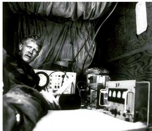
Author in "mini-wanigan" containing 30 MHz radar transmitter, receiver, and oscilloscope
